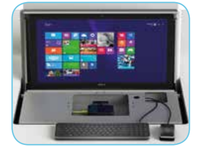
Keyboard tray with detail of Raspberry Pi mounting
